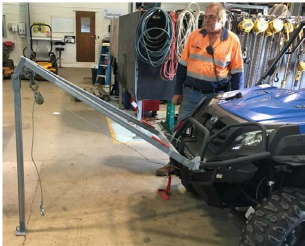
Col Johnson and his clever drillhole-casing puller.
